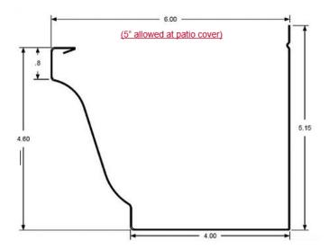
A. Exception: In patio cover installations where a 'rafter bracket' is used, gutter width can be modified to 5 inches to accommodate 'rafter bracket'. See Standard 34: Patio and Balcony Governos
