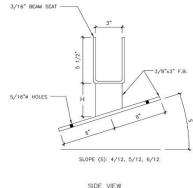
C. Rafter bracket as manufacture by "Beam Lift" or approved equal.
